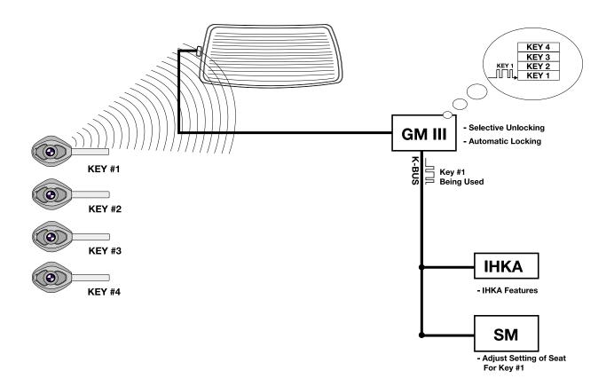
The key ID signal alerts the GM V to communicate with select control systems over the K Bus to store (when locked) or reset (when unlocked) certain driver adjustable settings.
